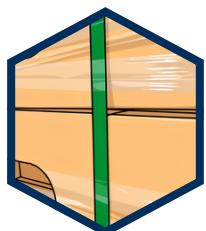
Strapping bands secure the load on the pallet.
